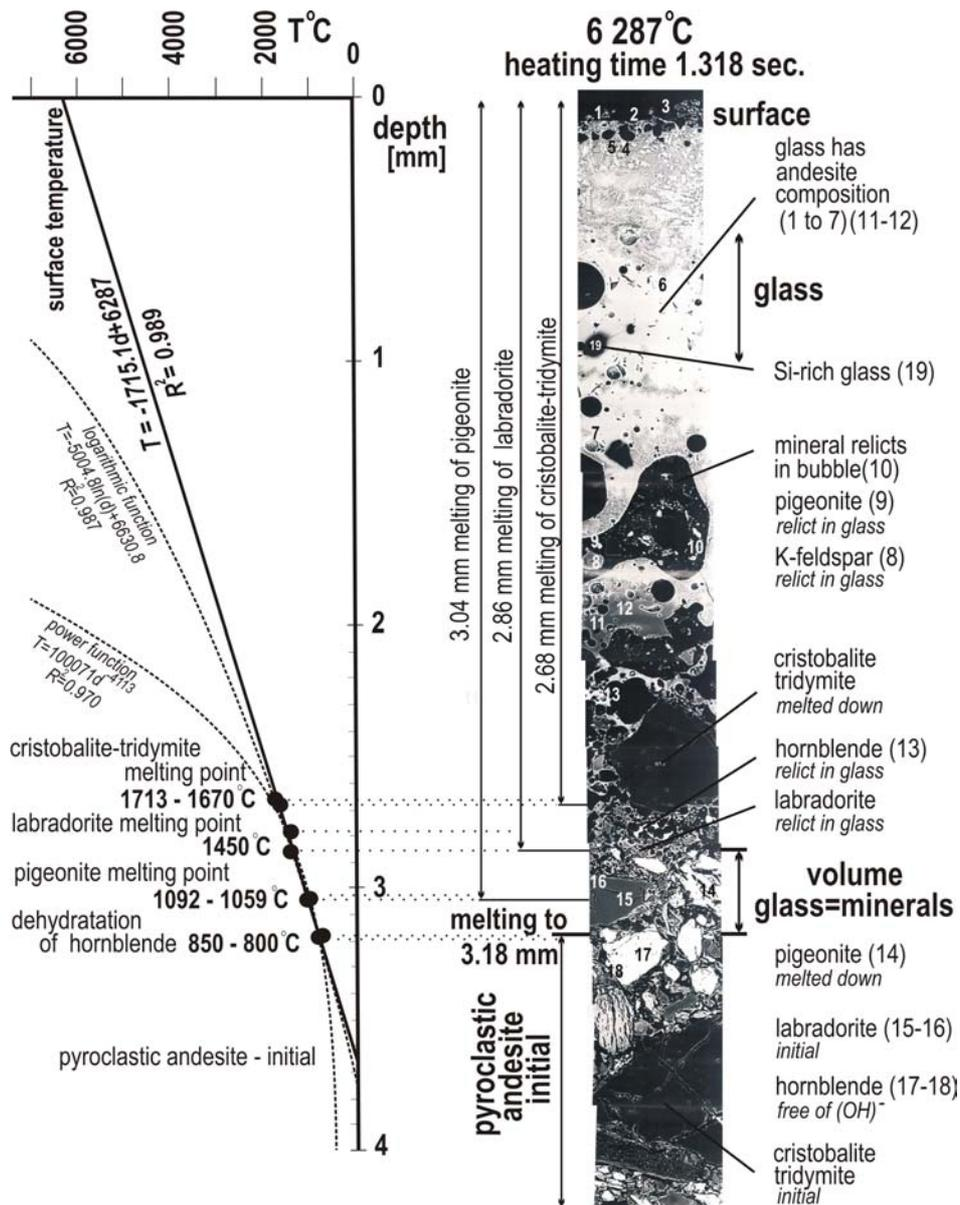
Fig. 3 Cross-section through melted pyroclastic andesite tile. The relations of average reached thickness of glass and original mineral assemblage. Backscattered electron image. The calculation of temperature 6287 °C on the tile surface was derived by the individual mineral relicts and surrounding melt, where temperature in the melt was falling by continual proportion in dependence of depth. 1 – 19 are the points of analyses.
