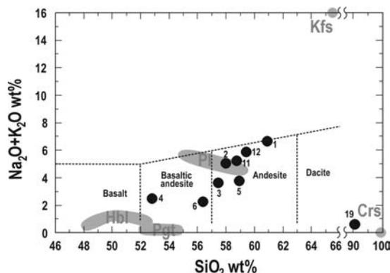
Fig. 2 Glass composition and hornblende (Hbl), pigeonite (Pgt), labradorite (Pl), K-feldspar (Kfs) and cristobalite-tridymite (Crs) and their compared compositions in diagram  $Na_2O + K_2O$  versus  $SiO_2$ . Andesite, basalt-andesite, and dacite fields are after the classification of volcanic rocks (Le Bas *et al.*, 1986). Analyses 1–6, 11–12, and 19 and their exact depths of positions are in Fig. 3.
