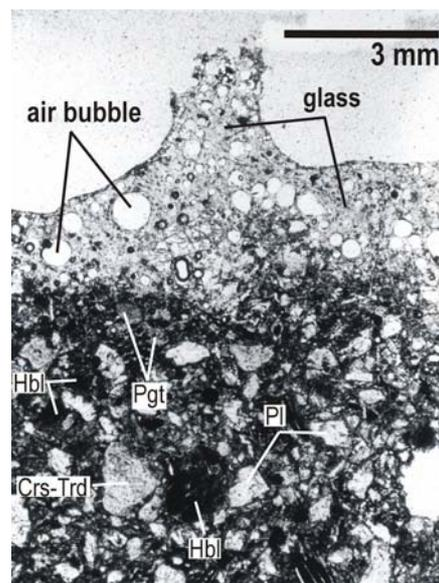
Fig. 1 Relationship between andesitic glass and mineral assemblage of the pyroclastic andesite tile in polarization microscope. Hbl – hornblende, Pgt – pigeonite, Pl – labradorite, Crs-Trd – cristobalite-tridymite.
